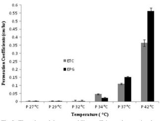
**Fig. 8.** The values of the permeability coefficients of acetaminophen through Eudragit RS films containing 20% TEC (ETC) or PEG 400 (EPG) at different temperatures
