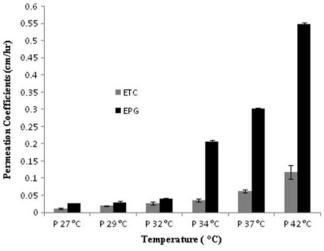
**Fig. 7.** The values of the permeability coefficients of propranolol hydrochloride through Eudragit RS films containing 20% TEC (ETC) or PEG 400 (EPG) at different temperatures
