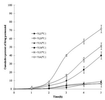
Fig. 3. The permeation of propranolol hydrochloride through Eudragit RS films containing 20% PEG 400 at different temperatures
