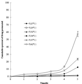
**Fig. 6.** The permeation of acetaminophen through Eudragit RS films containing 20% TEC at different temperatures
